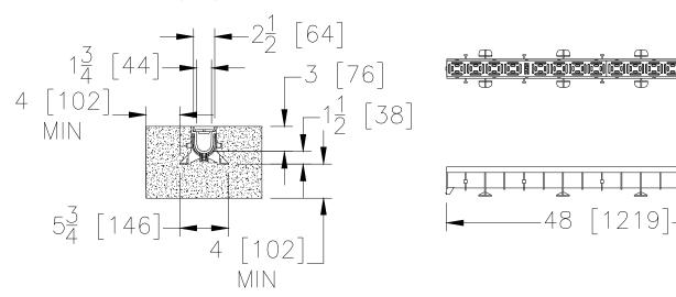
**ENGINEERING SPECIFICATION:** Zurn Z880 2 1/2 [64] Wide Trench Drain System shall be 48 [1220] long and 2 1/2 [63.5] wide. Drain shall be 3 [76] deep. Drain shall be made of (HDPE) High Density Polyethylene, and is UV-10 stabilized. Drain shall have bedding feet to be used for positioning and anchoring purposes. Drain shall have tongue and groove snap fit connection. Drain shall have 24 [610] long high-density polyethylene decorative grate (-POG) provided as standard.
